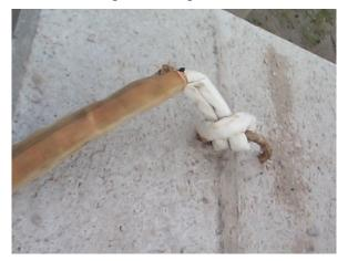
once it is locked on measure the line, attach a mooring ball, an ID tag and record in the spreadsheet of new moorings.
