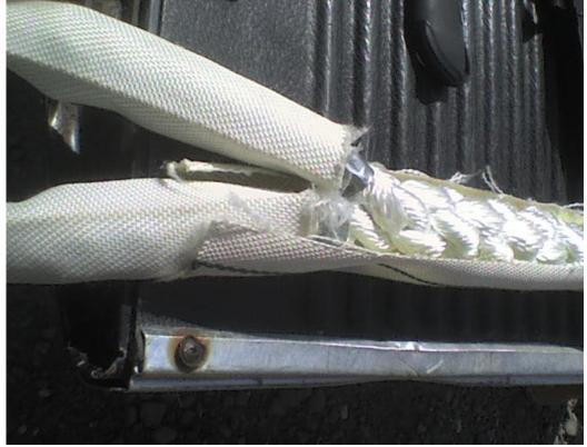
We also slid another piece of fire hose approximately 10 to 12 feet long over the hose from the other end. We slit the hose coming down over so that it would overlap the splice and reach down onto the fire hose in the eye splice, as shown in the picture above.
