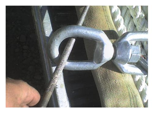
Once the swivel is smooth the eye spice is fed though the end without the nut and the eye splice is rolled over the top of the swivel and pulled down on itself like the picture below.
