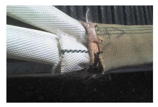
Once the chafe protection is in place we can work on the top end of the main mooring line.
