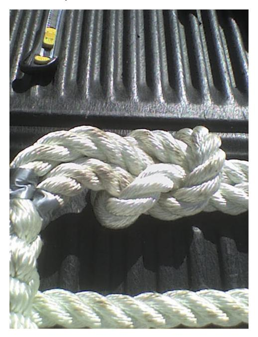
Neither end of the sacrificial line needs to be covered in fire hose. It will lock down tight enough that if you have to remove the two lines the easiest way to get them apart is to beat them with a rubber hammer. The top end of sacrificial line is then connected to the large swivel. This swivel should be checked for any ridges made in the manufacturing process, if there are any remove them with a small file.
